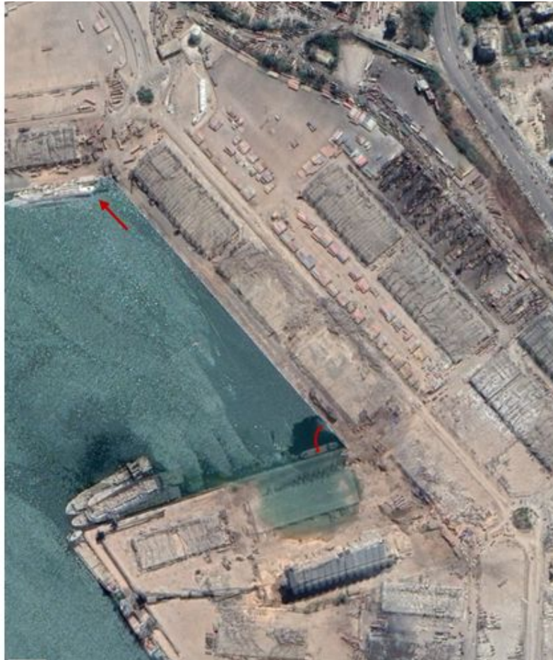
Figure 3.23. Superimposed Google Earth (™) images from 31 July 2020 and 5 August 2020. Straight arrow on the east side of Basin 3 shows the location of a capsized vessel (the Orient Queen). Curved arrow shows the before- and after-blast positions of a vessel washed up onto Quay 10 by the blast.
