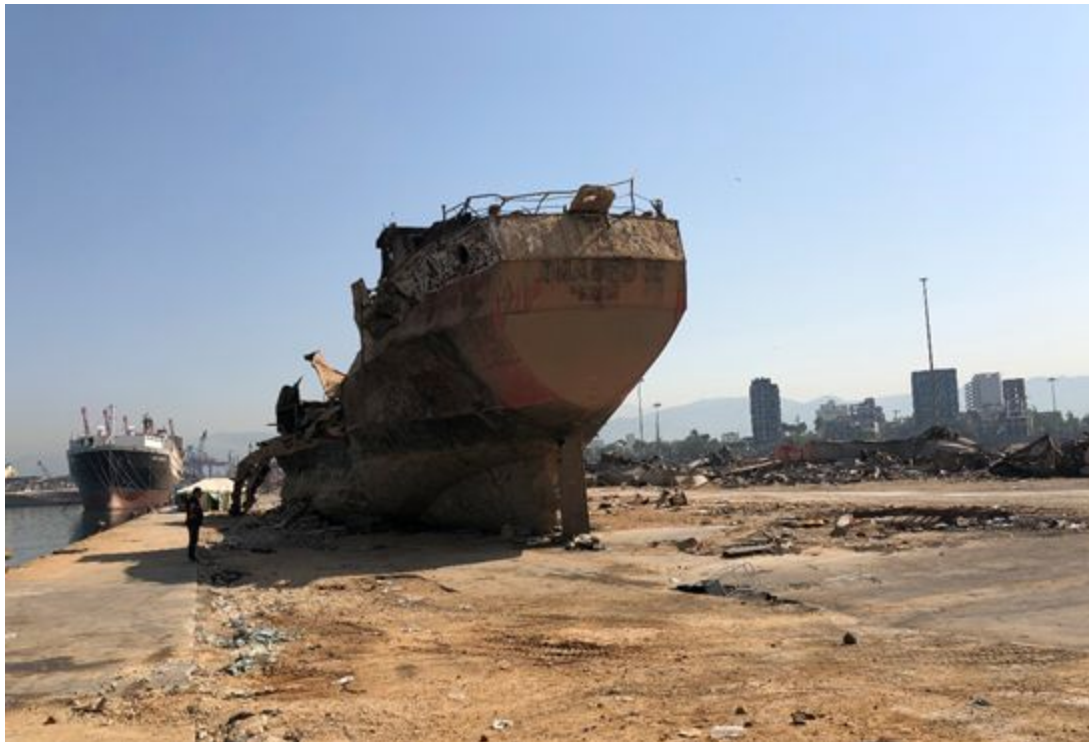
Figure 3.34. Medium-size vessel that was docked at Quay 9, lifted by the water wave generated by the explosion and left on the dock at Quay 10.( 33°54'3.04"N; 35°31'11.94"E).
