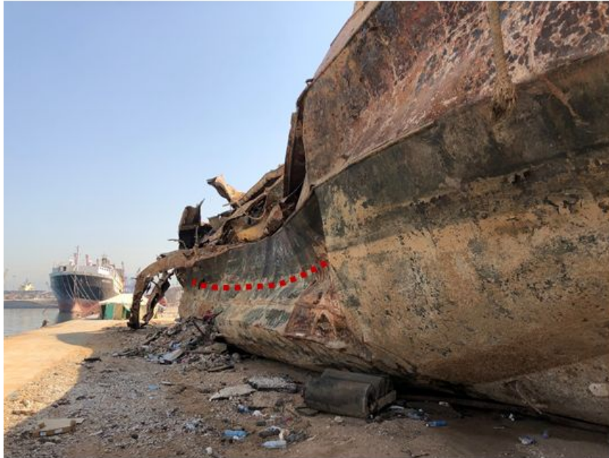
Figure 3.35. Closer view of the vessel with evidence of the indentation caused by the pressure wave. (33°54'4.13"N; 35°31'12.74"E).
