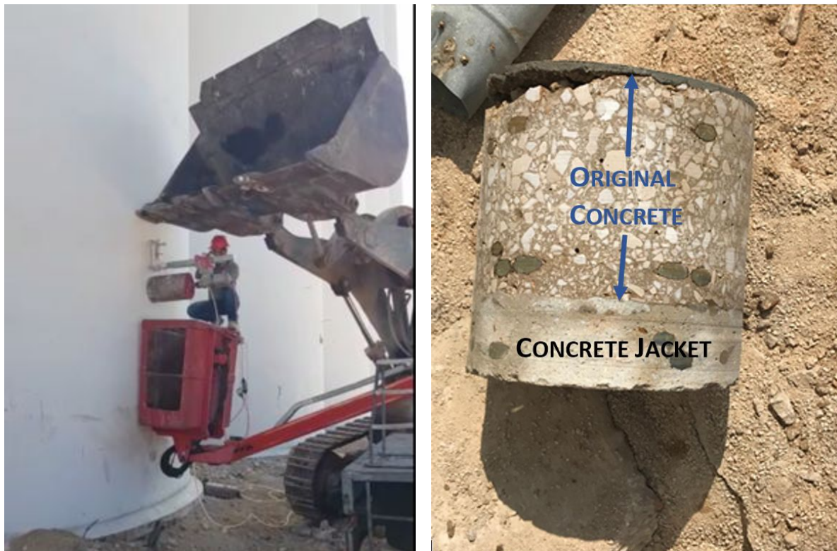
Figure 3.9. Coring through one of the “intact” cells. Note the improvised protection from falling debris from the damaged silo roof. The original concrete and the inner concrete jacket can be clearly seen in the recovered 30 cm core.
